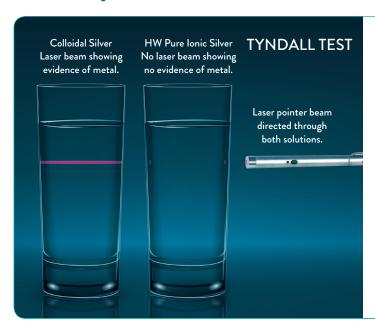
When a laser is shone through a liquid other than distilled water, a path of light can be seen similar to when you shine a torch through smoke or fog.
